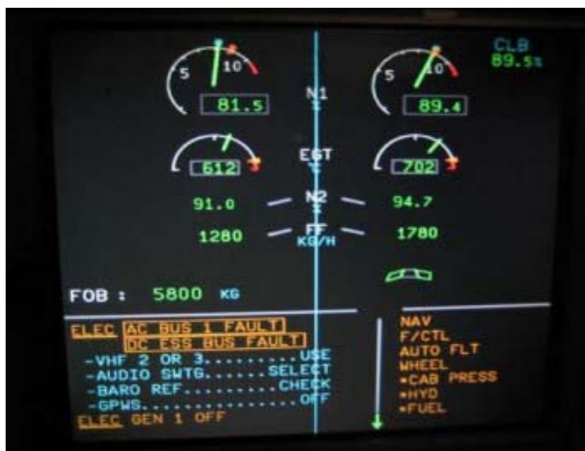
Figura 15: ECAM Actions A319
